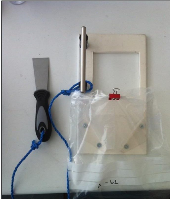
Figure 13.4.2: Wall scrape sampling device.
